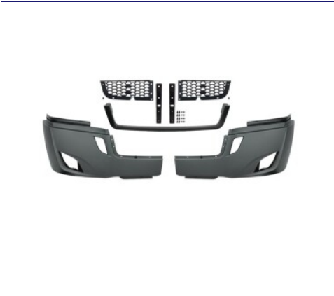
Item No. 21953 5-Piece Bumper Kit With Fog Light Opening For 2018-2023 Freightliner Cascadia MSRP: $ 606.79 OEM No. : 21-28981-002, 21-28980-004
